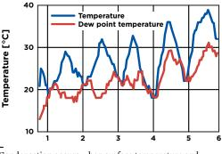
Condensation occurs when surface temperature and dew point temperature are equal.
