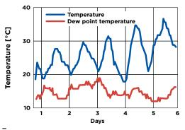
Dew point temperature is kept below surface temperature, preventing condensation and moisture damage.
