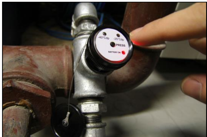
The DEWPOINT checker gives a clear indication of the conditions inside the equipment. The cup is screwed on the main body in order to protect the electronic components and offering IP rating IP67.
