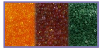
Water vapour can be seen being adsorbed by the silica gel desiccant at the orange/green interface and as it progresses through the adsorbent bed.
