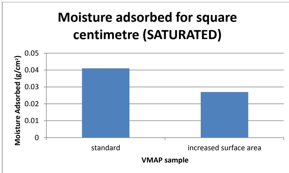
Figure 2 - Comparison between the two samples (moisture adsorption at 50%Rh and 22°C).
