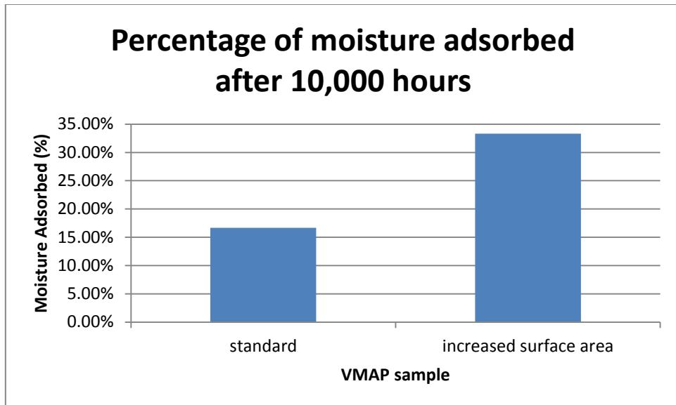
**Figure 1 - Comparison between the two samples (time of adsorption at 50%Rh and 22°C).**
